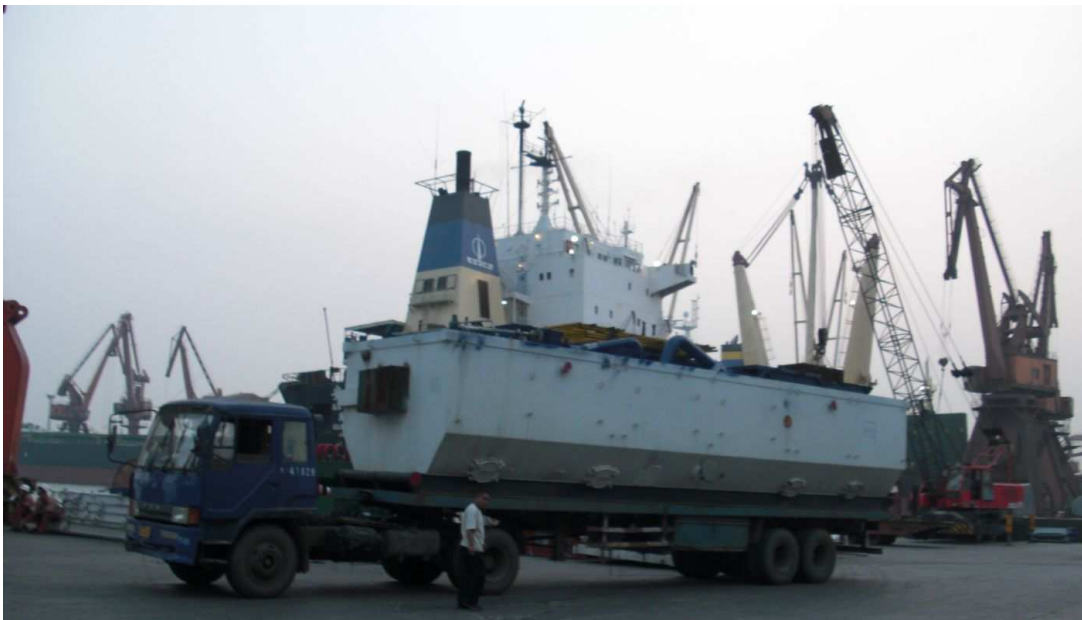
Photo 4 Mud circulation tank
